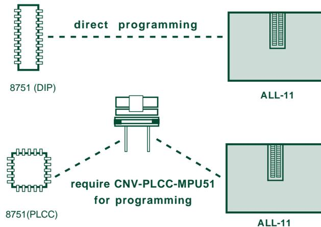
Some devices only come in surface mount packages like PLCC,PGA, SOP or have special programming requirements. These devices may also have higher pin counts from 44 pins to over 300 pins. These devices require an "adapter" to be programmed as well as an extra software driver. The software drivers are included with the adapters.
